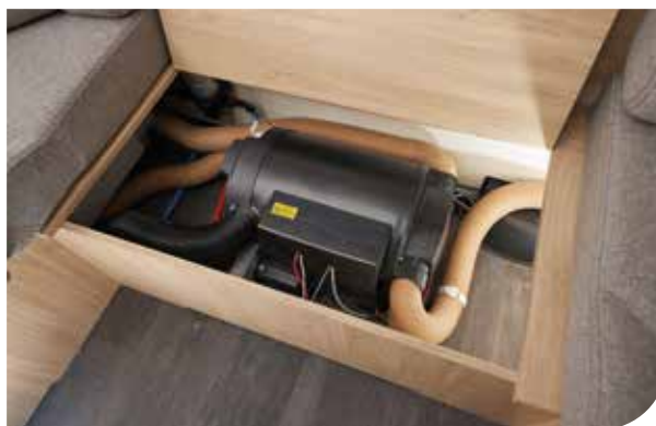
Heater/boiler (10L) TRUMA COMBI 6E (230V/GAZ)
